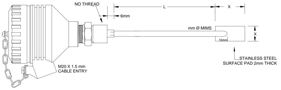
SUITABLE FOR USE WITH CERTIFIED Ex d / Ex e / Ex tD ENCLOSURE OR TRANSMITTER HOUSING WHICH HAS 1/2" NPT OR M20 X 1.5 MM PROCESS CONNECTION
